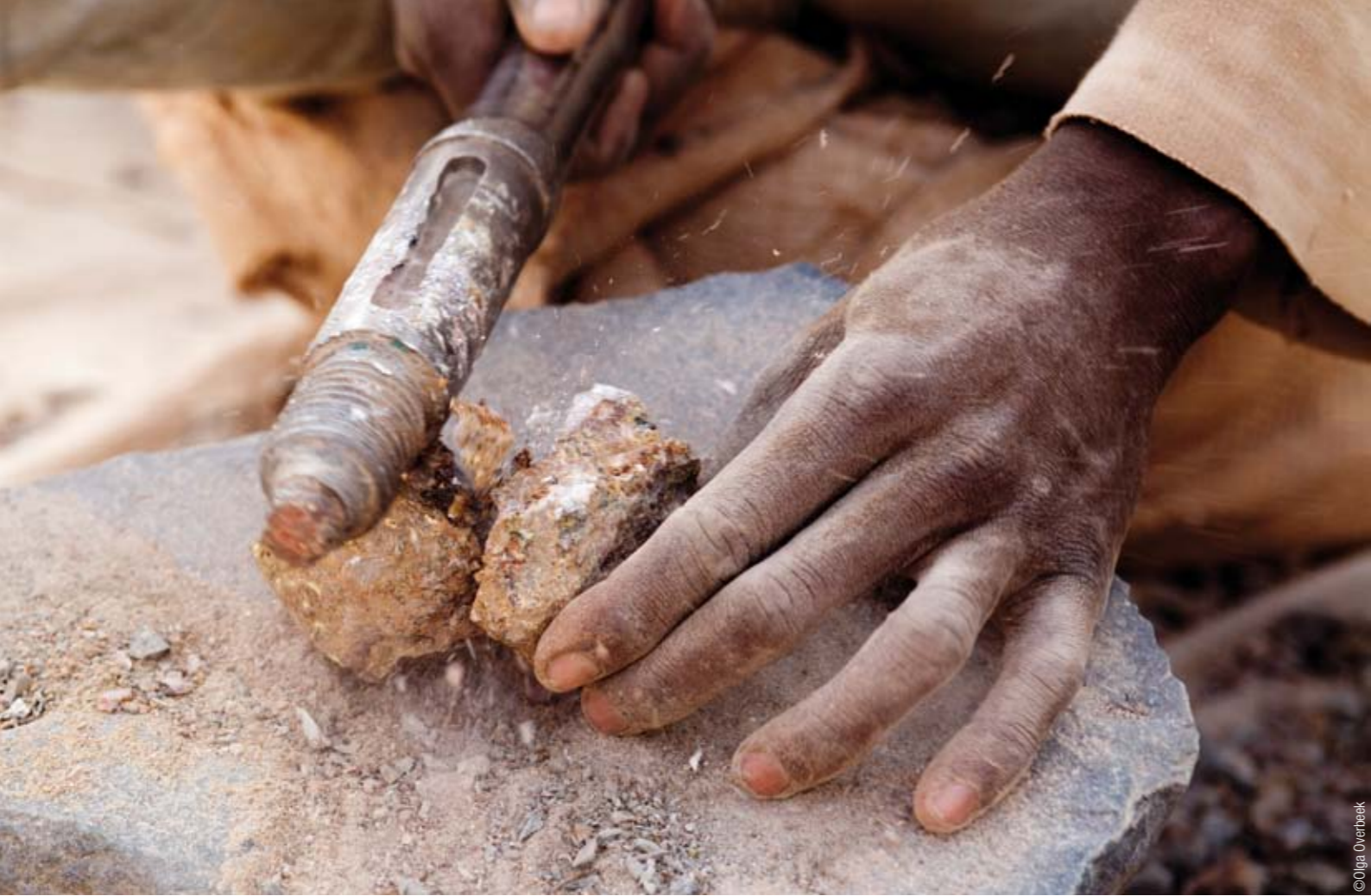
After stones are dug up from the mines they are brought to the gold processing site: stones are initially crushed so that they can go through the grinder (Bagega, Nigeria).
